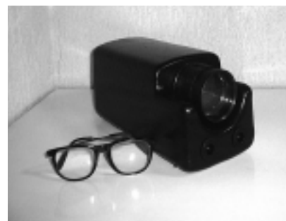
Fig. 2. The experimental model of optic electronic system for improving the visibility in smoke
