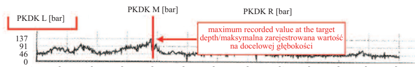
Fig. 7. Operating pressure registered during the formation of calibration column number D53 [20]
