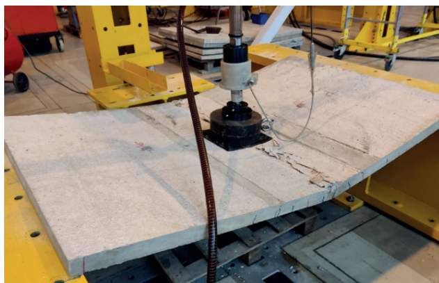
Photo 1. Repetitive failure for non-structural stay-in-place formwork by crushing the concrete
